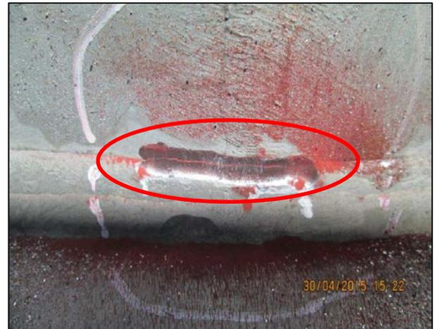
**Toe Crack Still Visible via MT Exam after Grinding**
